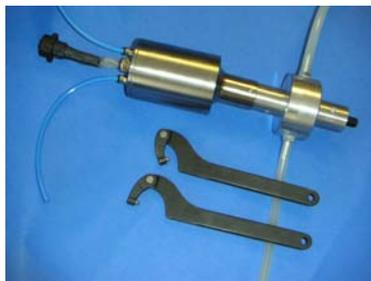
Water jacket with inlet-outlet silicone tubes
