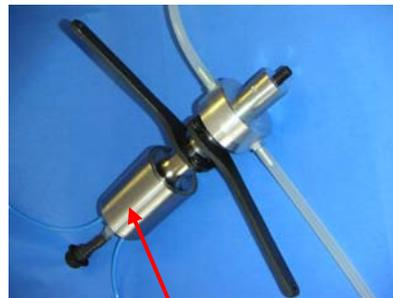
Do not fix anything to the converter housing (the housing is in elastic connection with the converter).
